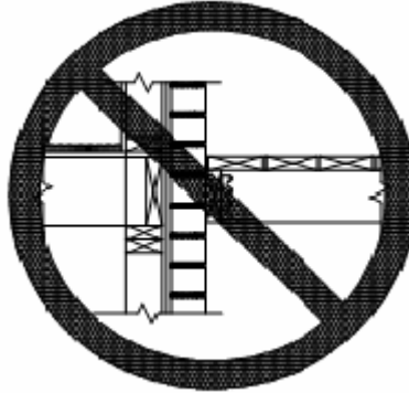
Direct to Masonry Veneer
