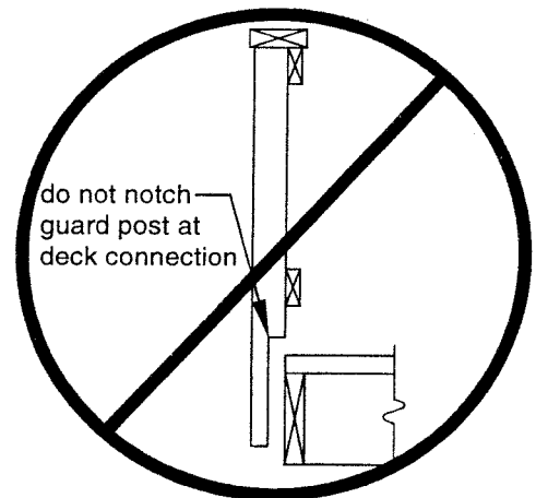
FIGURE 27: PROHIBITED NOTCHING AT GUARD POSTS
